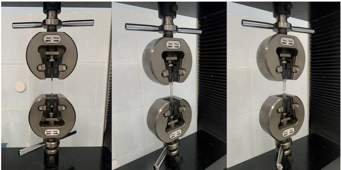
Figure 23 – Tensile tests of a standard specimen using the universal testing system
